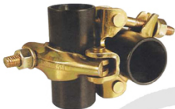
MI-001 DOUBLE COUPLER For Pipe OD 48.3 mm (EN-74 / BS-1139)
